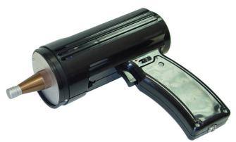
Sampling Device is intended for sampling of substances by pumping the air from the analyzed surface or volume through a concentrator.
