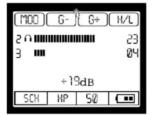
In addition to using the data displayed on the LCD screen, the operator may rely on audio signals from built-in speakers or headphones to define the presence of the second and third harmonics.
