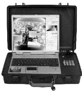
PC Based Control and Processing Unit
